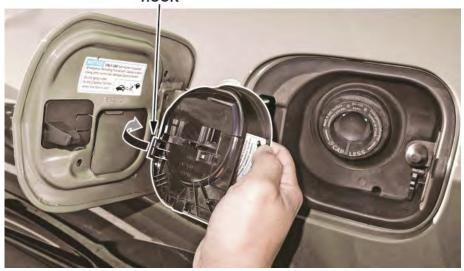
3. Press the left of the fuel lid cover to the fuel door until both locking tabs click. This indicates the fuel lid cover is securely and correctly installed.
