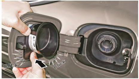
4. Make sure the fuel door closes and latches without contact or interference from the mis-fuel inhibit device and surrounding area. The gap between the door and the surrounding quarter panel should remain consistent.
