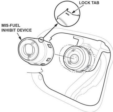
3. Install the new mis-fuel inhibit device.
