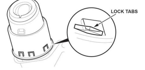
2. Pry up the lock tab and remove the mis-fuel inhibit device.
