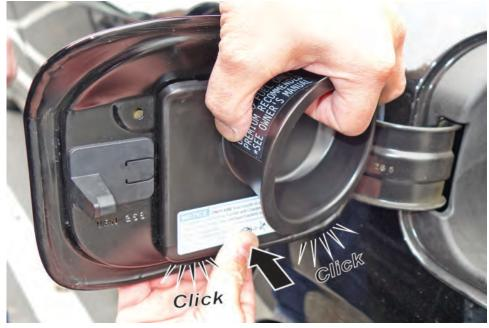
4. Make sure the fuel door closes and latches without contact or interference from the mis-fuel inhibit device and surrounding area. The gap between the door and the surrounding quarter panel should remain consistent.
