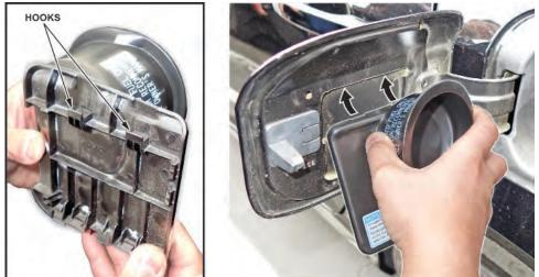
3. Press the bottom of the fuel lid cover to the fuel door until both locking tabs click. This indicates the fuel lid cover is securely and correctly installed.
