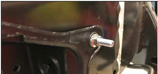
c) Install Frame Seal with Predrilled Hole w/o Weld Nut
