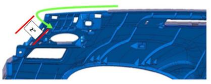
6) Working from one side, pull the adhesive backing and **CAREFULLY** apply the new foam cushion to the cleaned top front edge of the IP. Pull the backing off as you go. This will make the part easier to manage and reduce the chances of getting contamination in any exposed adhesive.
