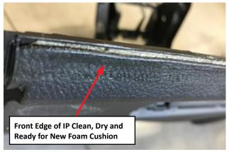
5) Before starting to apply the new foam cushion, leave 50mm (2") to wrap around the end and into the dash speaker area as shown in green in the illustration below. Be sure to not cover any holes.
