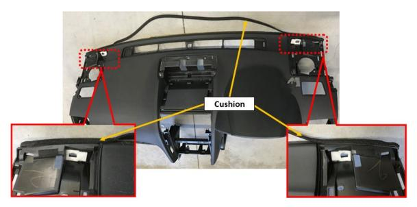
3) With the IP removed, CAREFULLY peel any remaining foam cushion / adhesive.
