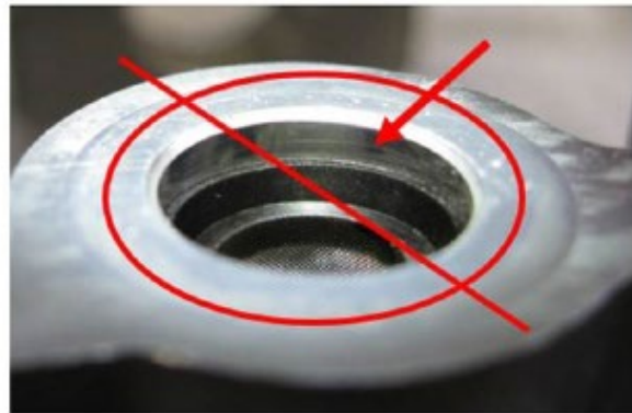
NG- Filter Screen installed too deep into the camshaft carrier bore.
