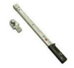
Torque Wrench 1332 40-200 Nm -VAG1332-(or equivalent)
