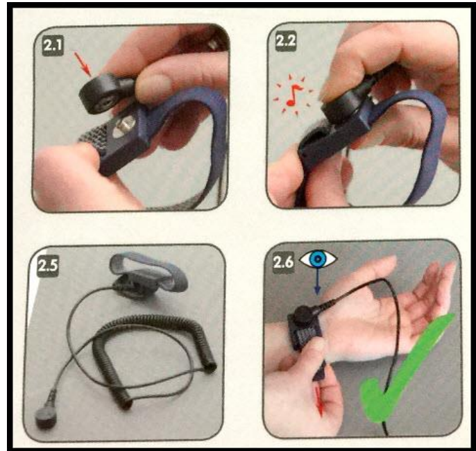
Figure 3. VAS6613 ESD work surface grounding wrist strap.
