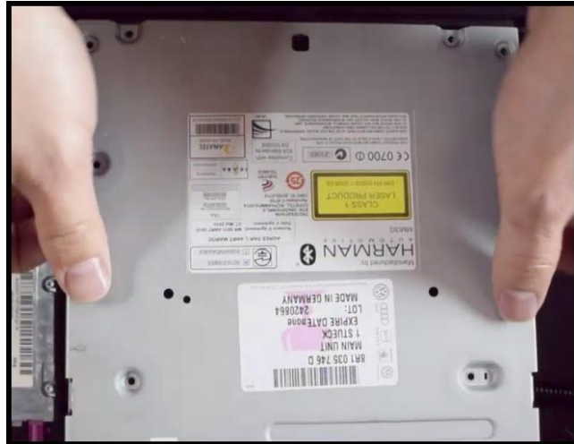
Figure 7. Pry top cover off with fingers.
