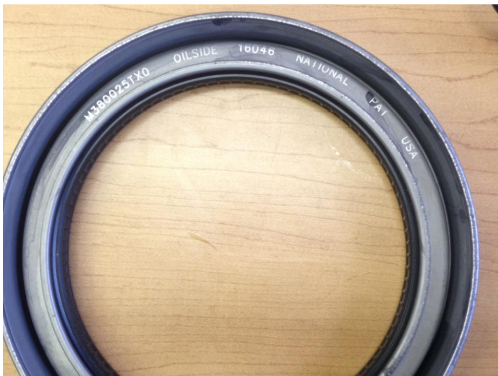
Figure 2: M380025TX0 NON OE seal – NO UT inscription on oil side
