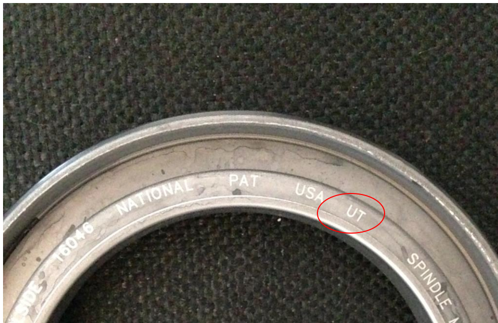
Figure 1: UT Inscription on Utility OEM seals – Oil side
