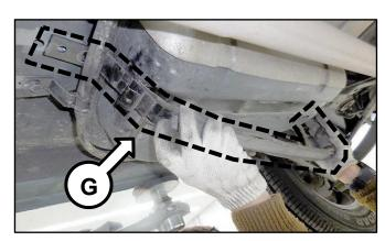
8. Before installing the new strap, clean the surface of the fuel tank strap area using a wire brush, and then spray the fuel tank surface where the strap will be placed with anti-corrosion undercoating spray. (Picture is for reference only, shows sprayed area after strap replacement)
