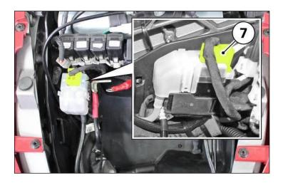
36) Place the battery into the battery compartment.
