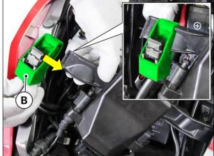
42) Install the BBS control unit support bracket/battery and tighten M5x0.8 retaining screw (1) to a torque of 5 Nm ± 10%.
