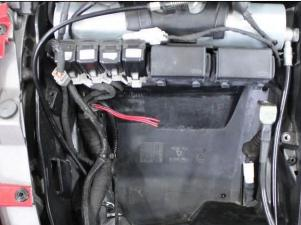
9) Remove the sheath at the ends of **red-yellow cable (11)** and **black cable (12)** for a total length of 10 mm / .4 in.
