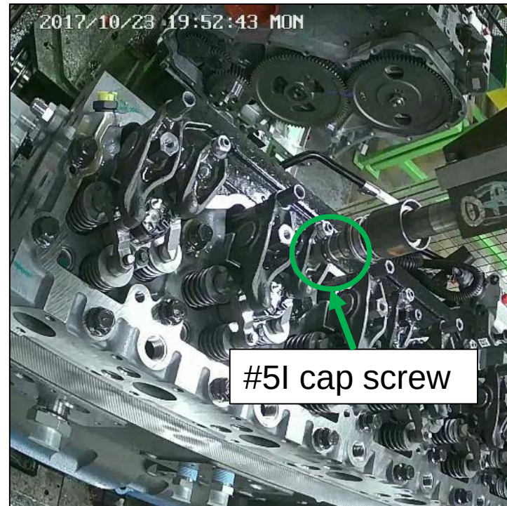
Video from 10/23 shows the c/s receiving torque
