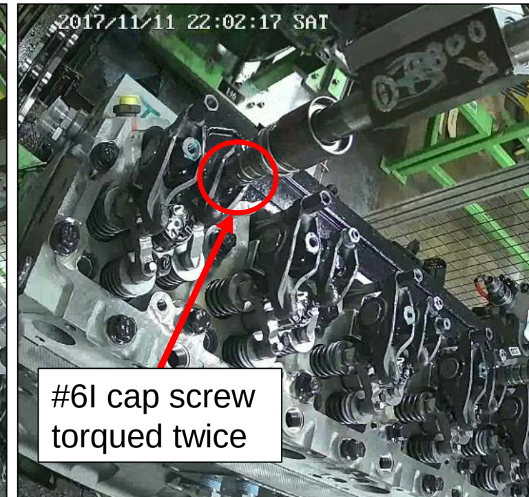
Video from 11/11 shows the c/s not receiving torque
