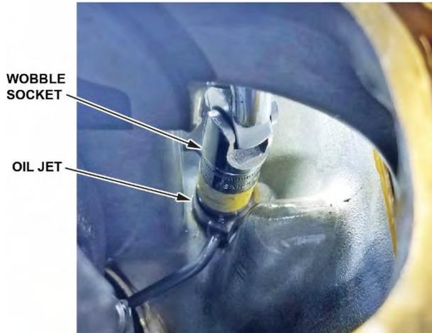
Here is an example of an improperly placed oil nozzle assembly. You can see the index hole is not filled by the nozzle alignment pin.
