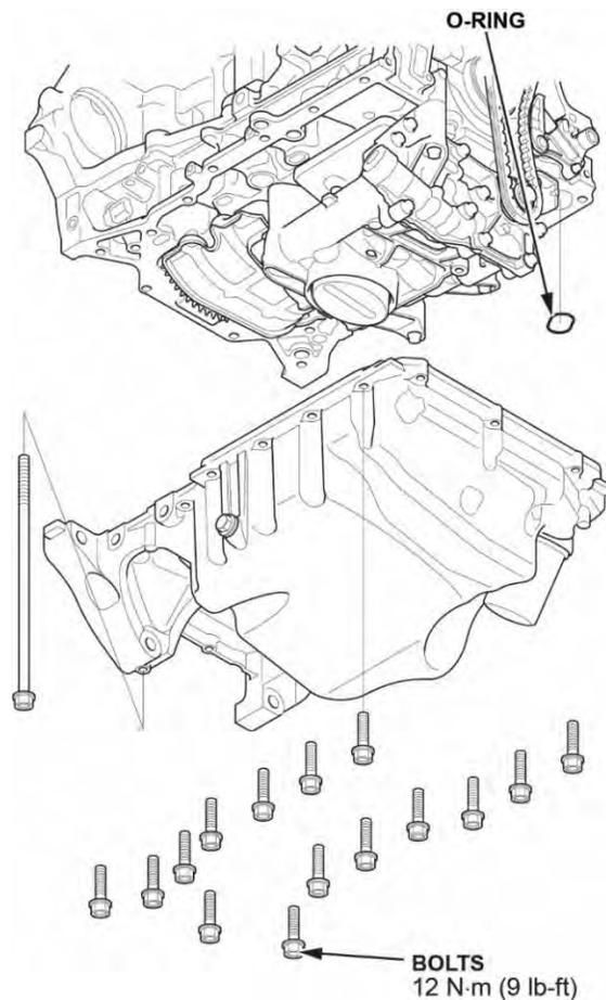
3. Tighten the bolts in three steps. In the final step, torque all bolts, in sequence, to **12 N·m (9 lbf·ft)**. Wipe off the excess liquid gasket on the each side of crankshaft pulley and flywheel/drive plate.
