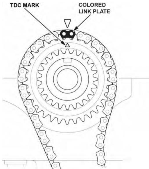
8. Set the oil pump chain on the oil pump chain sprocket with the punch mark aligned with the center of the colored link plate.
