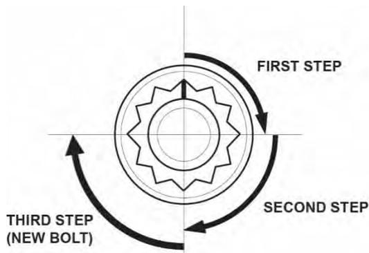
NOTE: Remove the cylinder head bolt if you tightened it beyond the specified angle, and go back to step 6 of the procedure. Do not loosen it back to the specified angle.
