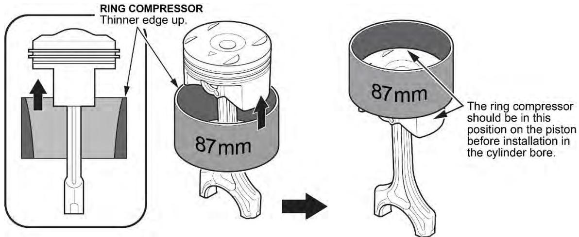
6. Set the ring compressor on the cylinder bore, then push the piston in with your hands.
