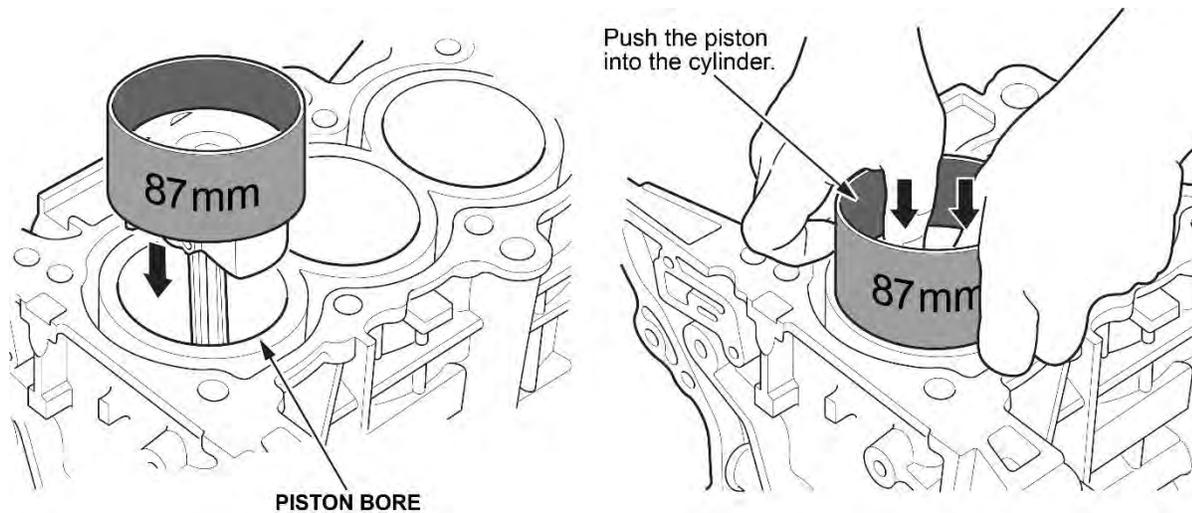
7. Stop after the ring compressor pops free, and check the connecting rod-to-rod journal alignment before pushing the piston into place.
