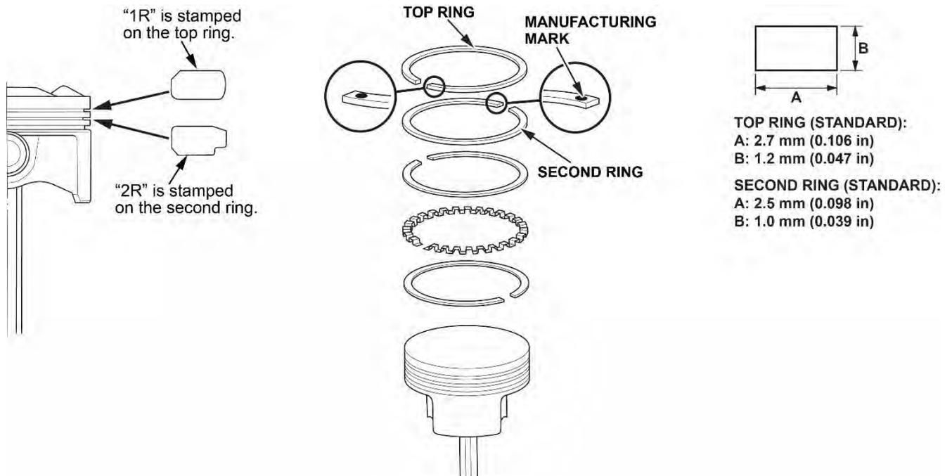
2. Rotate the rings in their grooves to make sure they do not bind.
