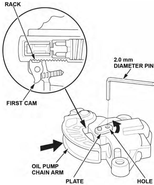
10. Install the oil pump chain auto-tensioner.
