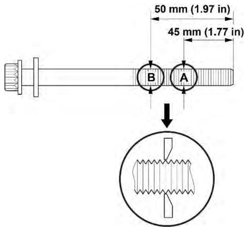
8. If either diameter is less than 10.6 mm (0.417 in), replace the cylinder head bolt.
