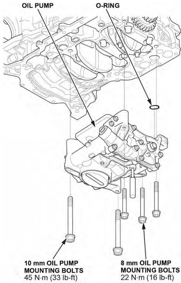
6. Tighten the oil pump mounting bolts.
