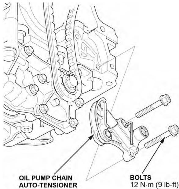
11. Remove the pin from the oil pump chain auto-tensioner.
