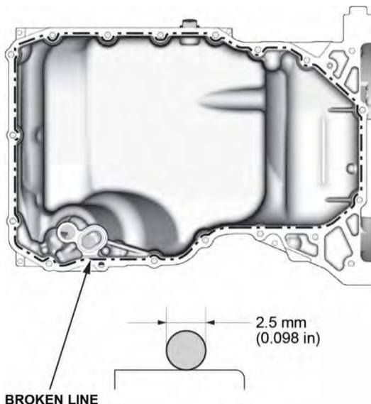
2. Install the oil pan with a new O-ring.
