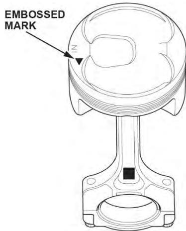
5. Set the piston in the ring compressor and position it in the cylinder, noting the rod/cap marks that you made in step 3 of REMOVAL OF PISTONS AND RODS.
