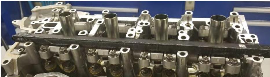
14. Remove the cylinder head bolts. To prevent warpage, loosen them in sequence 1/3 turn at a time. Repeat this sequence until all of the bolts are loosened.
