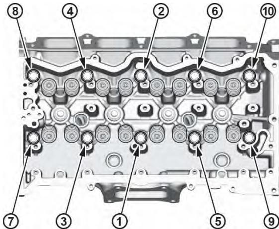
11. After torquing, tighten all cylinder head bolts in two steps (90 degrees per step) using the sequence shown in step 10. If you are using a new cylinder head bolt, tighten the bolt an extra 90 degrees.
