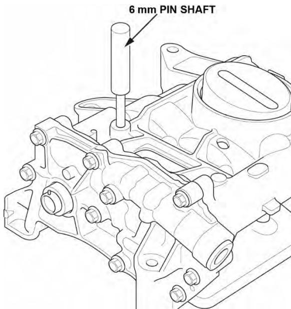
5. Apply new engine oil to the threads of the oil pump mounting bolts, then loosely install the oil pump with a new O-ring.
