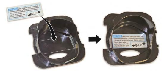
5. Make sure the clamps engage the fuel fill door, then slide the lid away from the fuel fill door hinge. Press on the lid until the clips snap into place. This indicates the lid is secured and correctly installed.
