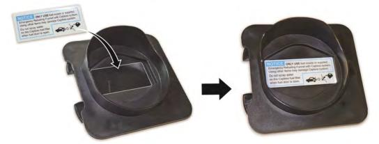
5. Make sure the clamps engage the fuel fill door, then slide the lid cover away from the fuel fill door hinge. Press on the lid until the clips snap into place. This indicates the lid is secured and correctly installed.
