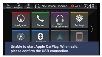
If you get a vehicle in your shop for this, be aware there's no available solution at this time. So, don't try replacing the head unit; it won't make a difference. For now, as a workaround, just do a battery cable reset.
