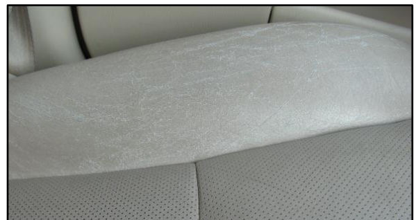
Figure 3. Wear Caused by Outside Influence
