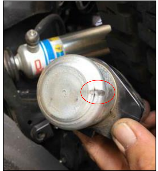
Figure 4. Plating Damage Example
