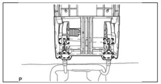
c) Disconnect the 4 cable clamps on each handle..
