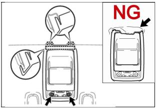
b) Engage the 3 guides and install the 2 screws on each handle.
