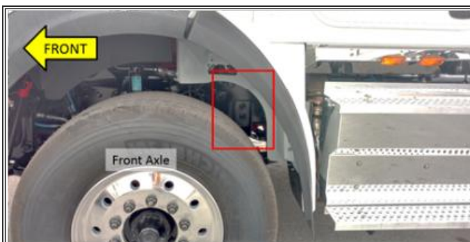
Figure 1: Location of Frame Tie
