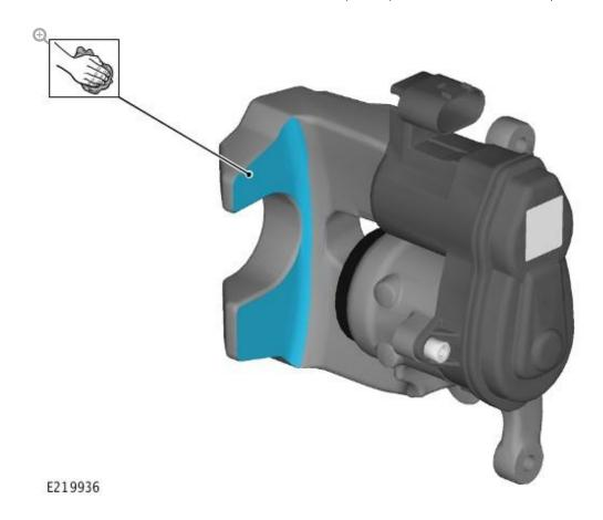
When cleaning the rear brake caliper make sure the contact area for the outboard rear brake pad is clean and free from contaminants.
