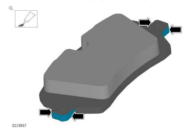
Apply Molykote Cu- 7439+ to the rear brake pad contact areas.
