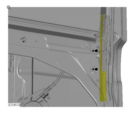
Install the rear left door window seal into the channel.
