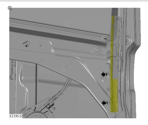
Release the rear left door window seal from the channel.
