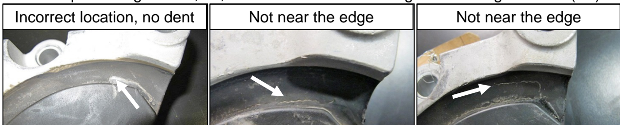
Marks above are commonly mistaken as dent/scratch but are GOOD.
