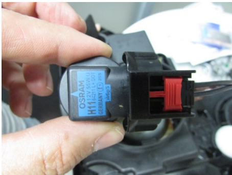
Figure 3 Clip not engaged / Clip engaged
