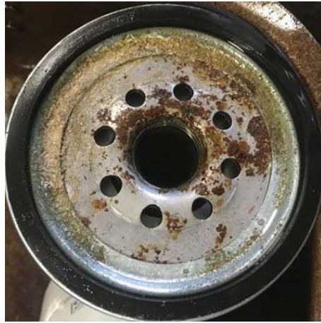
Crystal buildup and corrosion/rust present on primary filter
