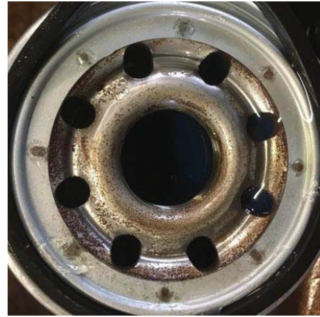
Corrosion/rust on secondary filter
