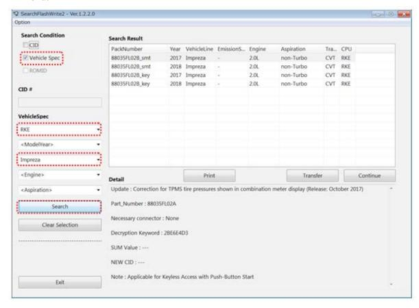
• Reprogram the RKE control module following the normal FlashWrite procedure.
