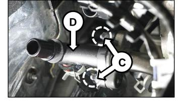
4. Be sure to remove and discard the old "brown" ATF warmer connector pipe Oring that may still be attached to the engine side of the heater pipe. The new ATF warmer connector will have a new "blue" O-ring attached to install.
