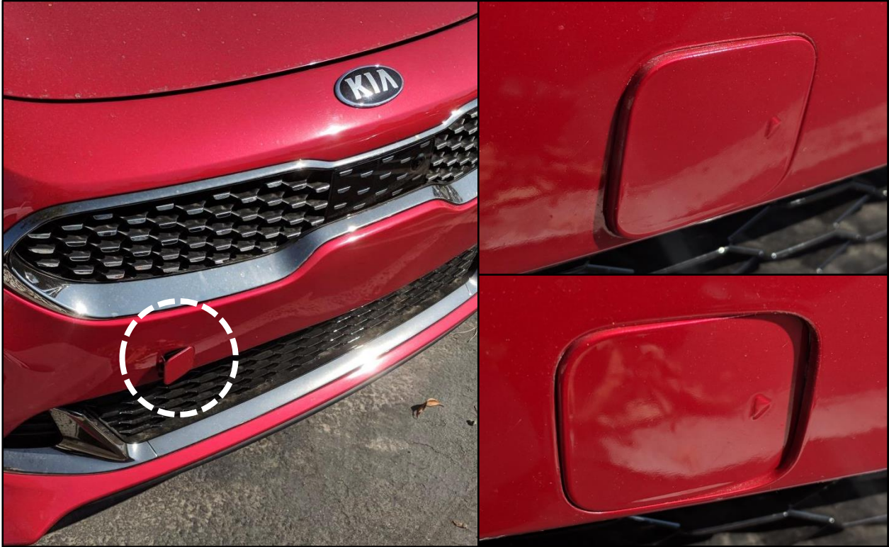
INCORRECT SAMPLES: Tow Hook Cap not properly inserted and not flush with front bumper cover.
