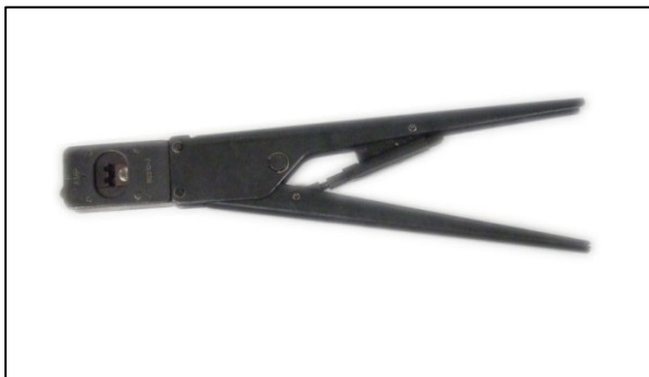
Figure 3: 682254 Amp crimper (For optional repairs)
