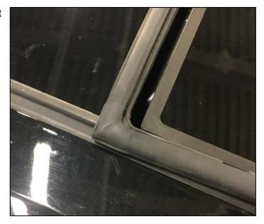
6. Start by installing the end of the seal.
