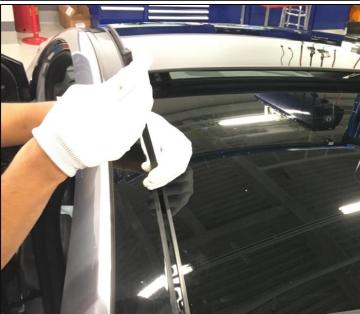
2. With the panoramic roof rear glass seal fully removed, lay out the replacement seal to prepare for installation.
