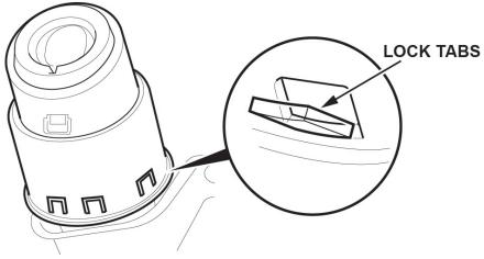
2. Pry up the lock tab and remove the mis-fuel inhibit device.
