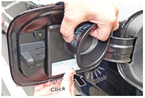
7. Make sure the fuel door closes and latches without contact or interference from the mis-fuel inhibit device and surrounding area. The gap between the door and the surrounding quarter panel should remain consistent.
