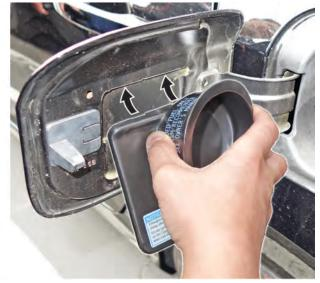
6. Press the bottom of the fuel lid cover to the fuel door until both locking tabs click. This indicates the fuel lid cover is securely and correctly installed.
