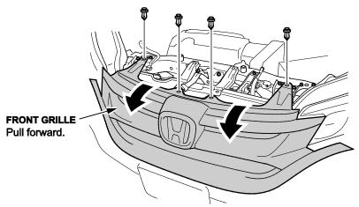
2. Remove the four clips from the front grill and slide the upper duct forward and remove it.
