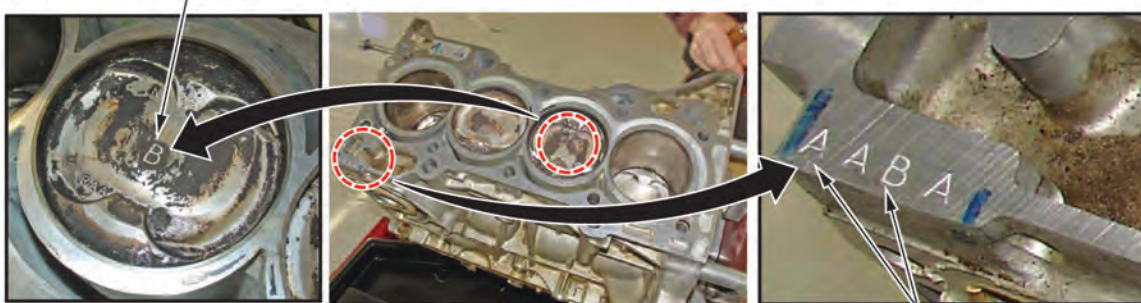
The "A" and "B" represents piston size. Piston sizes can be mixed in an engine block assembly.
