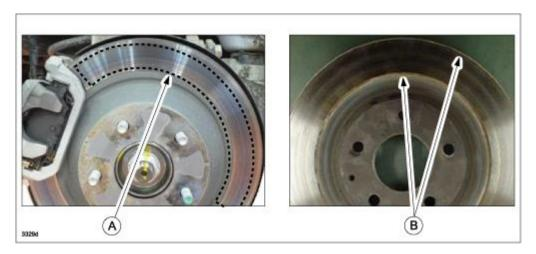
6.Inspect the brake pads for whitened by heat (A) or abnormal wear on only the outer pad (B) due to brake dragging.
