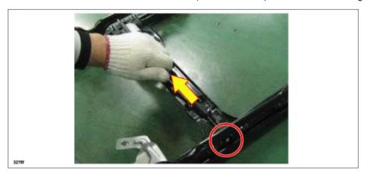
**CAUTION:** If the new cable is bent too much during installation, operational noise may occur. DO NOT hold the new cable around the ends.
