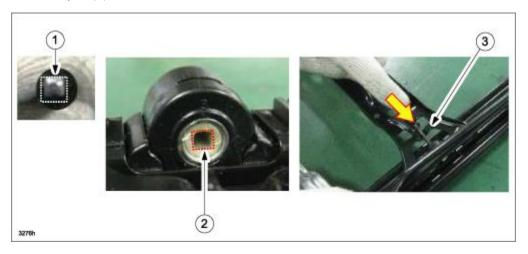
**CAUTION:** If the cable is bent too much during installation, operation noise may occur. DO NOT hold around the tip of the cable.
