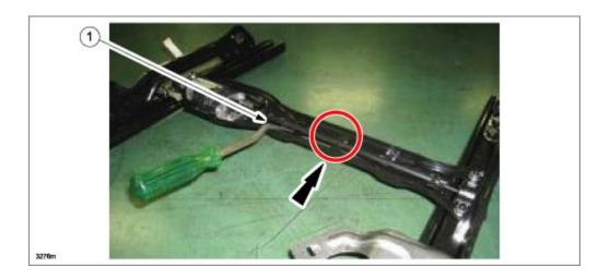
**CAUTION:** After removing the cable, DO NOT operate the slide switch, otherwise, it may cause damage to the adjuster unit.
