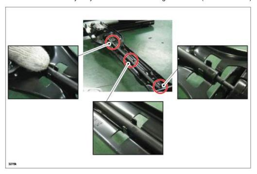
15. Look from under the seat and confirm the new cable is not bent, curved or floating.
