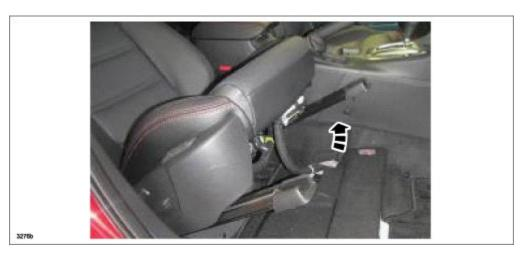
7. Insert a screwdriver between the frame and the cable (shown in the red rectangle below).
