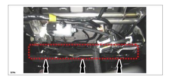
8. Using the screwdriver (1), release the center cable fixing point, as shown below.
