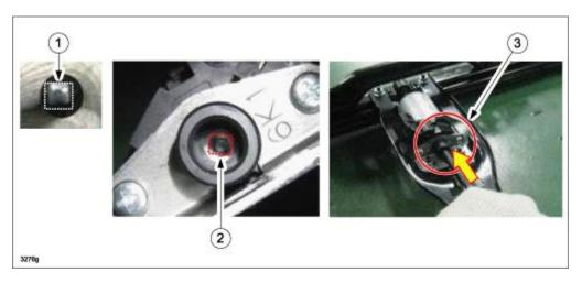
13. Align the square tip of the new cable (1) with the square shape of the gear box (2) and push the cable all the way in (3).
