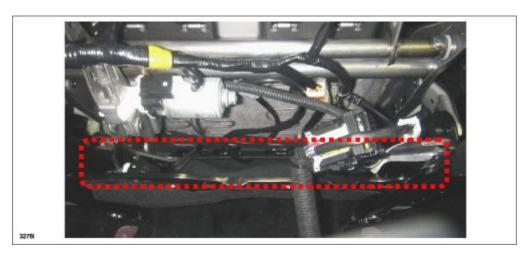
16. Check the installation of the cable to the motor and to the gear box (1) and the installation of the cable along the frame (2).
