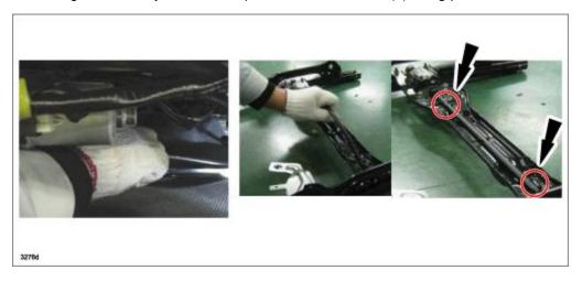
**CAUTION:** When removing the cable, remove it from the motor side first. If it is removed from the gear box side first, the engagement position could be misaligned.
