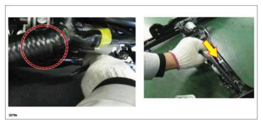
11. Pull the cable in the direction of the arrow (as shown below) to remove it from the gear box.
