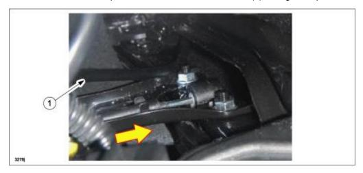
14. Press the cable firmly in by hand and secure it along the bracket (as shown below).
