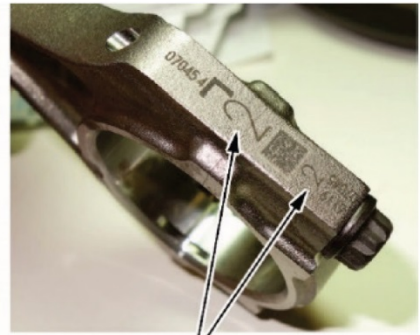
These are manufacturing marks, and do not indicate the cylinder number.
