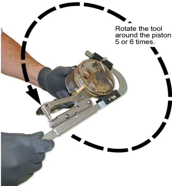
7. Remove the piston groove cleaning tool and clean off the carbon from the tool bit.
