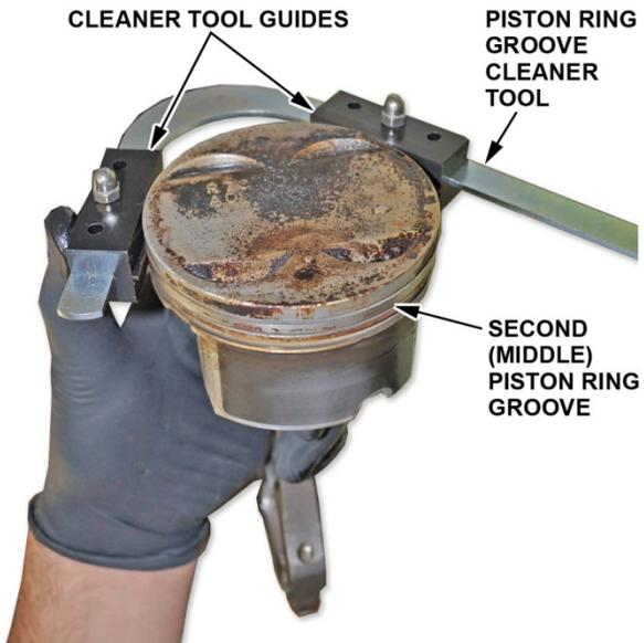
4. Press the handle on the piston ring groove cleaner tool and slide the cleaning bit onto the appropriate piston ring grooves.
