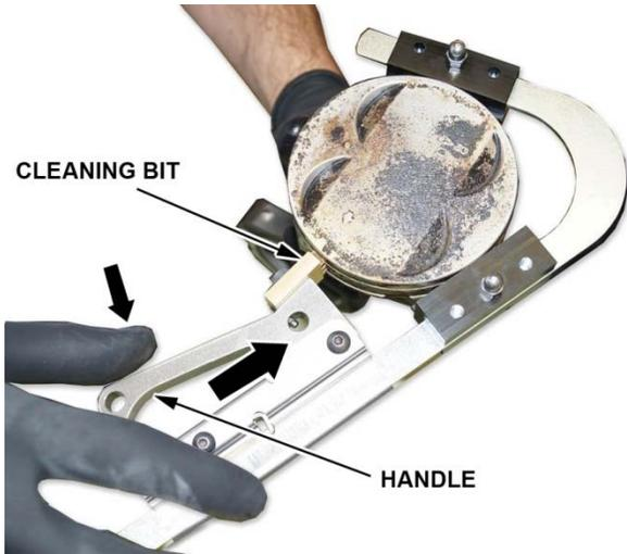
5. Once the cleaning bit is in the appropriate ring grooves of the piston, make sure the tool handle clicks in to place.
