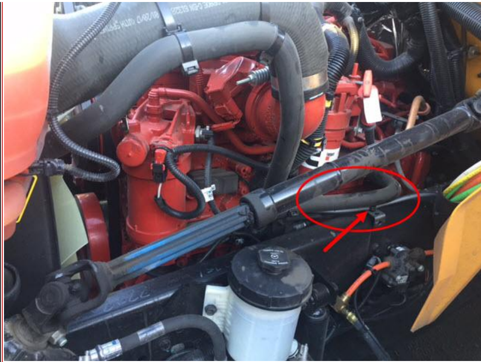
Figure # 1 Air Compressor Inlet Hose
