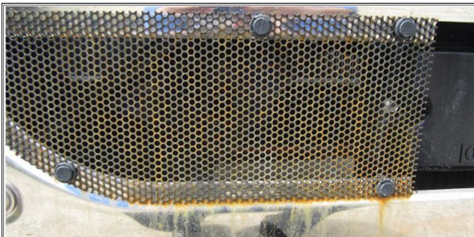
Figure #1: Rust/Corrosion on the Front Bumper Rock Guard
