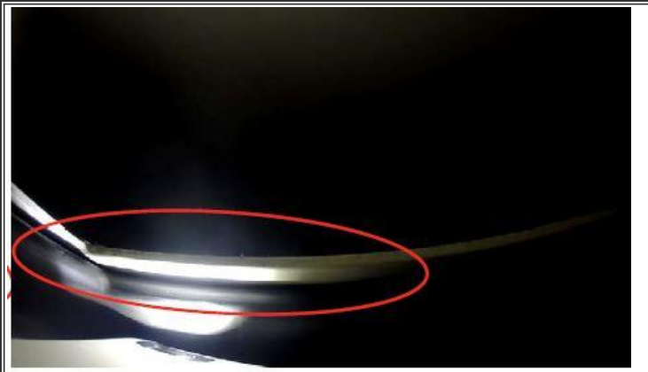
Figure 2: Hood misaligned with respect to Boot seal
