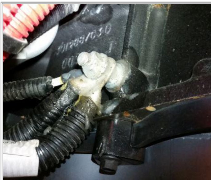
Figure 1: Ground cable connection
