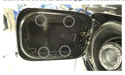
6. Installation of the fuel lid cover is the reverse of removal. Verify all the tabs are engaged, and slide the cover away from the fuel door hinge until it clicks. This indicates the fuel lid cover is secured and correctly installed.
