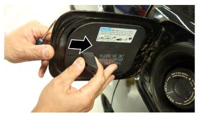
5.3. Slide the cover until the four tabs disengage from the slots in the fuel door.
