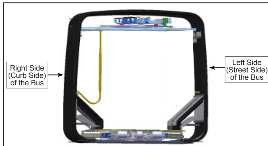
Figure 2 - Typical View of Articulation System Inside the Vehicle
