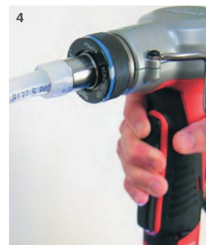
Expansion with Milwaukee M12 ProPEX Expansion Tool
