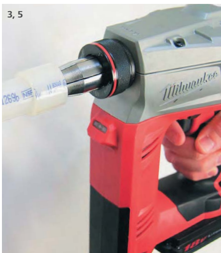
Expansion with Milwaukee M18 ProPEX Expansion Tool
