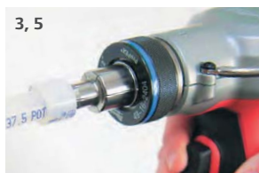
Expansion with Milwaukee M12 ProPEX Expansion Tool
