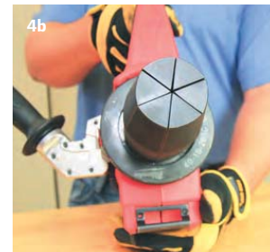
Correct Expansion Head Alignment
