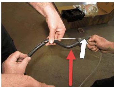
Water Drain Hose Bends — Work the tool gently in the area of the bends.
