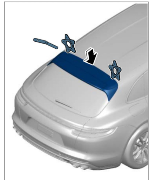
Checking gap dimensions
