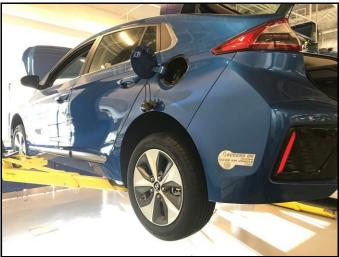
11. Remove the rear driver's side wheel by removing the 5 lug nuts.
