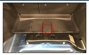
7. Wear insulated protective gloves and disconnect the high voltage safety plug by following the illustration steps shown to the right.
