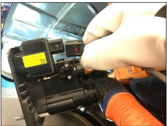
Use a T15 Torx screwdriver to remove the two screws holding the charging lock/unlock actuator.
