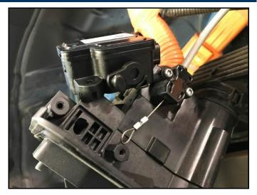
18. Remove the red rubber seal from the old part and place it onto the new part.
