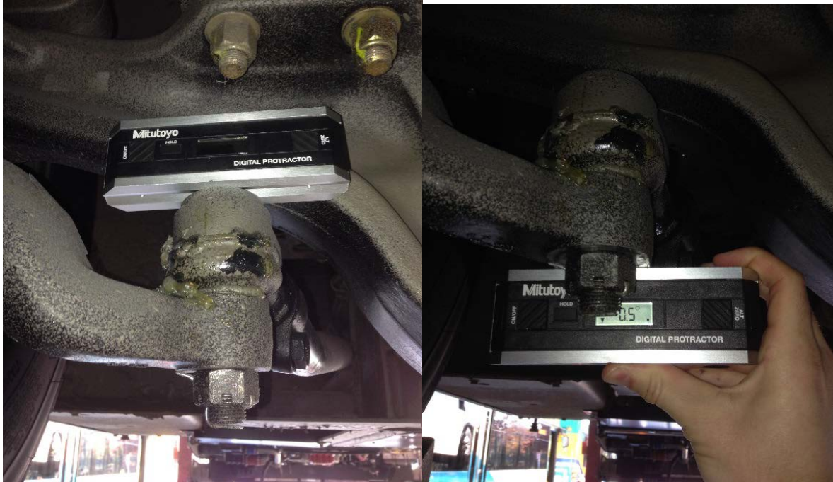
Figure 3 – Side to side Draglink Angle Measurement. Using a digital protractor, reference the top of the draglink by placing the protractor on top of the socket and zeroing it out; then place the protractor on the machined surface of the steer arm adjacent to the draglink. This angle should be less than 2 degrees. The pictures above are from a 35'/40' draglink, but the same principle applies to the 29' draglink.
