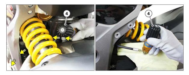
5) Mark the pre-load adjustment pipe with a marker at a distance of 60 mm starting from the **union (5)** on knob side.
