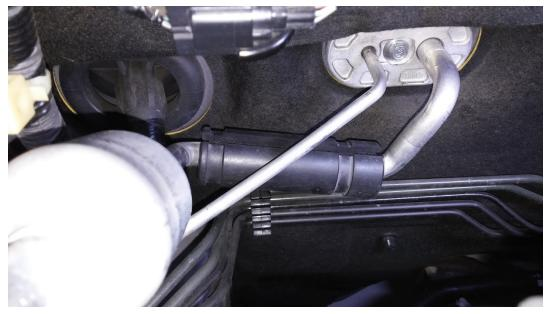
5. Secure the rubber hose with the 4 zip ties as shown below.
