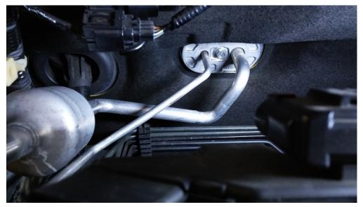
2. Wrap the pipe with one foam sheet as shown (long edge along the pipe).
