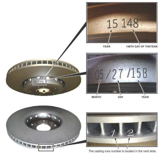
The casting core number is located in the vent slots.
