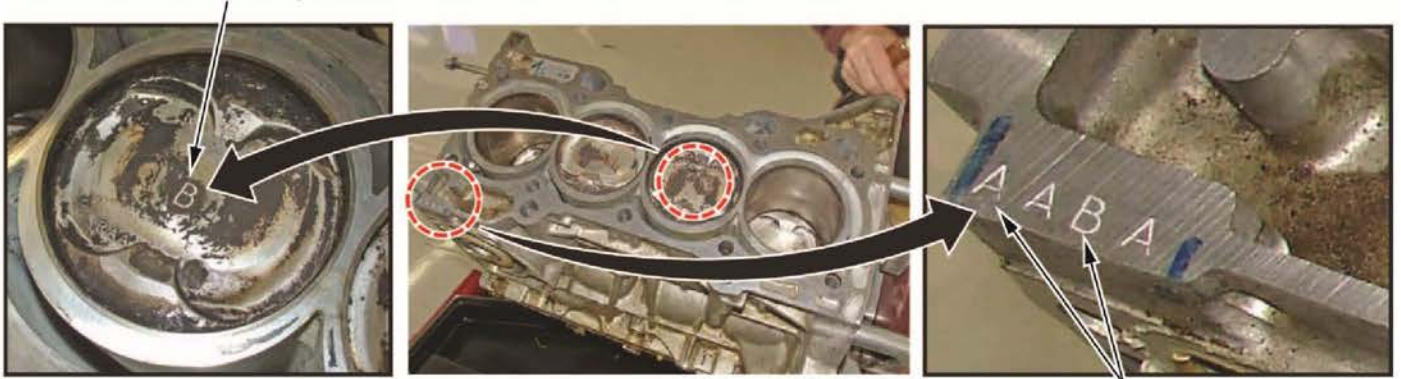
The "A" and "B" represents piston size. Piston sizes can be mixed in an engine block assembly.
