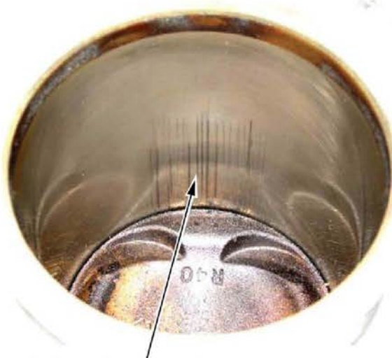
Light scratches are not abnormal. Ensure a fingernail or pencil "catches" on the scratches before replacing the block.
